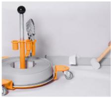
During assembly, the soft skirting is evenly rolled off the Easy Scooter. The protective paper of the adhesive tape must be removed and the profile glued to the wall. After this, press down completely with the Doellken rubber hammer.
