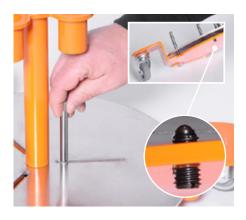
The guide and retaining pins are easily adjustable. If desired, the turntable can be braked by adjusting the screw on the underside of the device.
