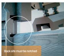
Close the clamping device and notch. Use Döllken hot melt to fix the end caps
