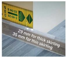
Lock the clamping device and put the mark to the border of the lay-on surface...
