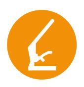
1 Turn over the profile on the head - put it straight on the trestle - lock the clamping device - cut very carefully.
